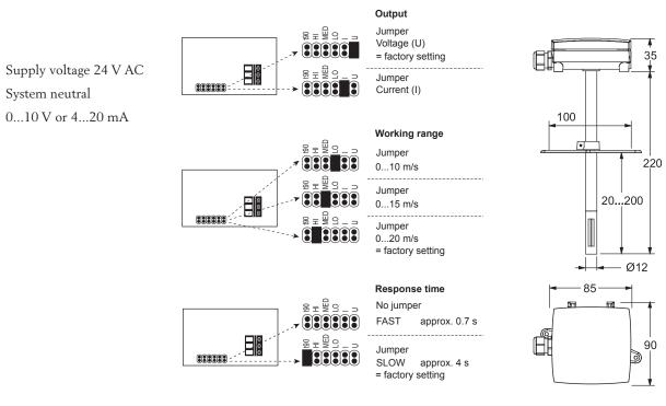
The output signal, working range and response time are selected via the jumpers according to the picture.
