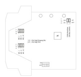
Configuration of position feedback: If a feedback signal is connected to the module, the jumper is to be configured for a feedback signal accordingly.
