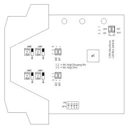
Configuration of position feedback: If a feedback signal is connected to the module, the jumper is to be configured for a feedback signal accordingly.
