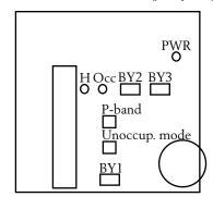
Jumper BY1 Right = Internal sensor (factory setting)
